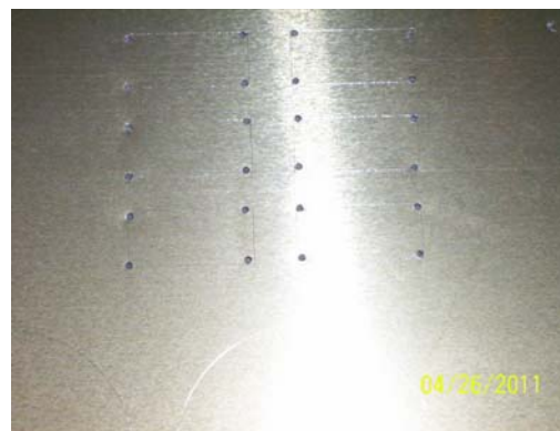
Holes drilled for locating corners
