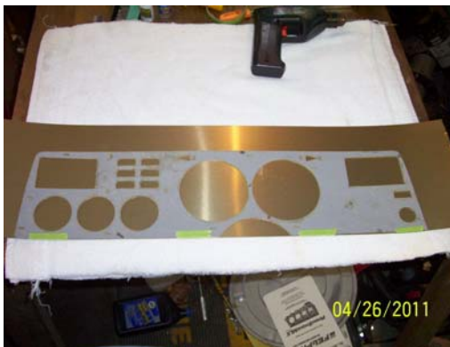
Template taped in place
