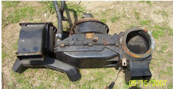
***You need to remove nine clips from the heater box that hold the two halves together. Once the box is split the core can be removed.***
