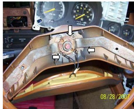
*First you need to remove two screws that hold the horn pad to the wheel. Next remove the two wires that make the horn work. To remove these all you need to do is pull gently on the connectors and the horn pad is now off the wheel. Next use a 15/16" socket to remove the nut that holds the wheel to the column.*
