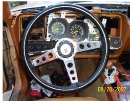
*Next reconnect the horn wires and reinstall the horn button and the installation is now complete. Next article will be on checking the dash lights for proper operation.*
