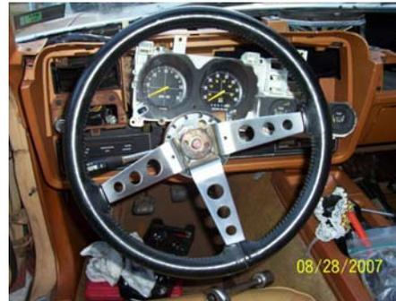
*Carefully make sure that the new wheel is oriented in the correct position and install it on the column and replace and tighten the nut. Be sure that the nut is properly tightened or the wheel could come loose and cause loss of steering control.*
