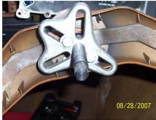
*Next install a steering wheel puller by using the two holes on the wheel. This centers the tool on the column and by turning the center bolt on the puller the wheel pops off easily. Once the wheel is removed it is time to install the new one.*
