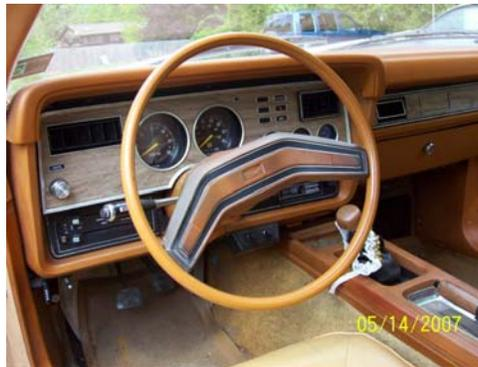
*This is the original steering wheel that was installed at the factory. Because the car is now 30 years old the vinyl on the wheel has faded and discolored to the point that it can not be brought back. So a factory sport wheel will be installed that still looks like new and is easier to maintain. Before beginning be sure front wheel are straight as this will assure the new steering wheel will be on straight when you're finished.*
